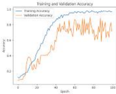
Fig. 10: Training and Validation Accuracy Trends Over Epochs for the LSTM model
